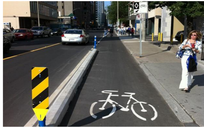
Fig.59. One-way roadway bicycle path, Montreal, Canada Source : The Centre of Active Transportation
