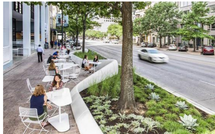
Fig.82. Green drainage bed, Congress Avenue, Austin, US Source : Kevin Michael Sullivan
