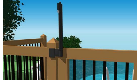
Figure 8 Example of a latch installed at 1.52m on the exterior of the enclosure
