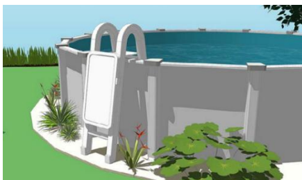
Figure 1 Example of a ladder equipped with a self-closing and self-latching gate
