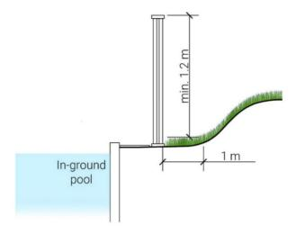
Where the enclosure is a chain-link fence, the mesh must have a maximum width of 30 mm. If slats are inserted in the mesh, their width may be greater than 30 mm but they must not allow the passage of a spherical object more than 30 mm in diameter.
