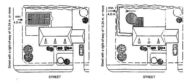
iii) These minimum distances are always measured from the water line, namely the imaginary line separating the edge of the swimming pool and the beginning of the water.
