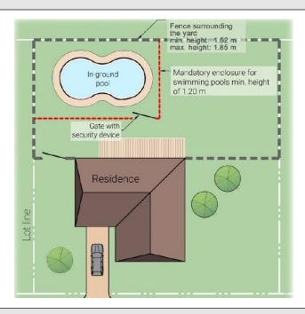
**FENCE preventing access to the pool from the home** (The safety gate must be equipped with self-closing and self-latching passive security device)
