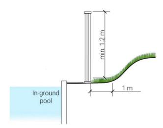
Example of calculation of the height of the enclosure
