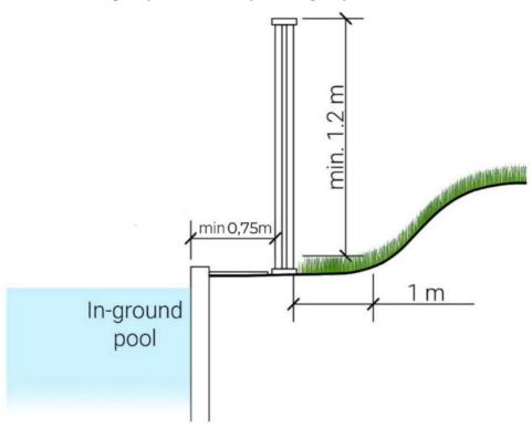
Example of calculation of the height of the enclosure
